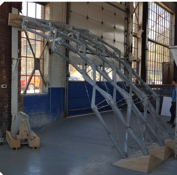
Axon of our PETG mold in a reconfigurable jig system with steel plates at each node to ensure precision.
